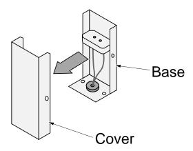
3. Insert the wires from the accent light through the gasket removed in step 1 then through the hole exposed in the burner tray. Attach the accent light base to the burner tray using the screws removed in step 1.
