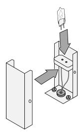
5. Remove the two screws holding the control cover in place.
