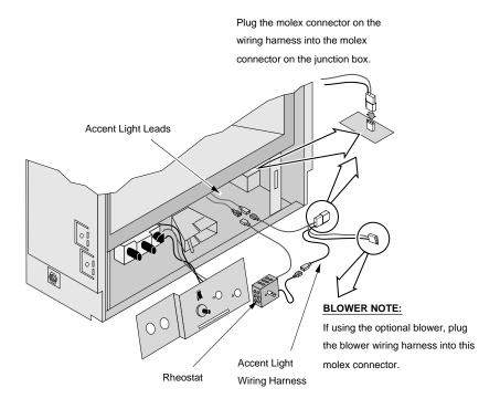
7. Attach the rheostat to the cover plate as shown below. Make sure the small white tab on the rheostat inserts through the corresponding small hole on the cover plate. Re-attach the cover plate, making sure all wiring is away from any hot or moving surfaces.
